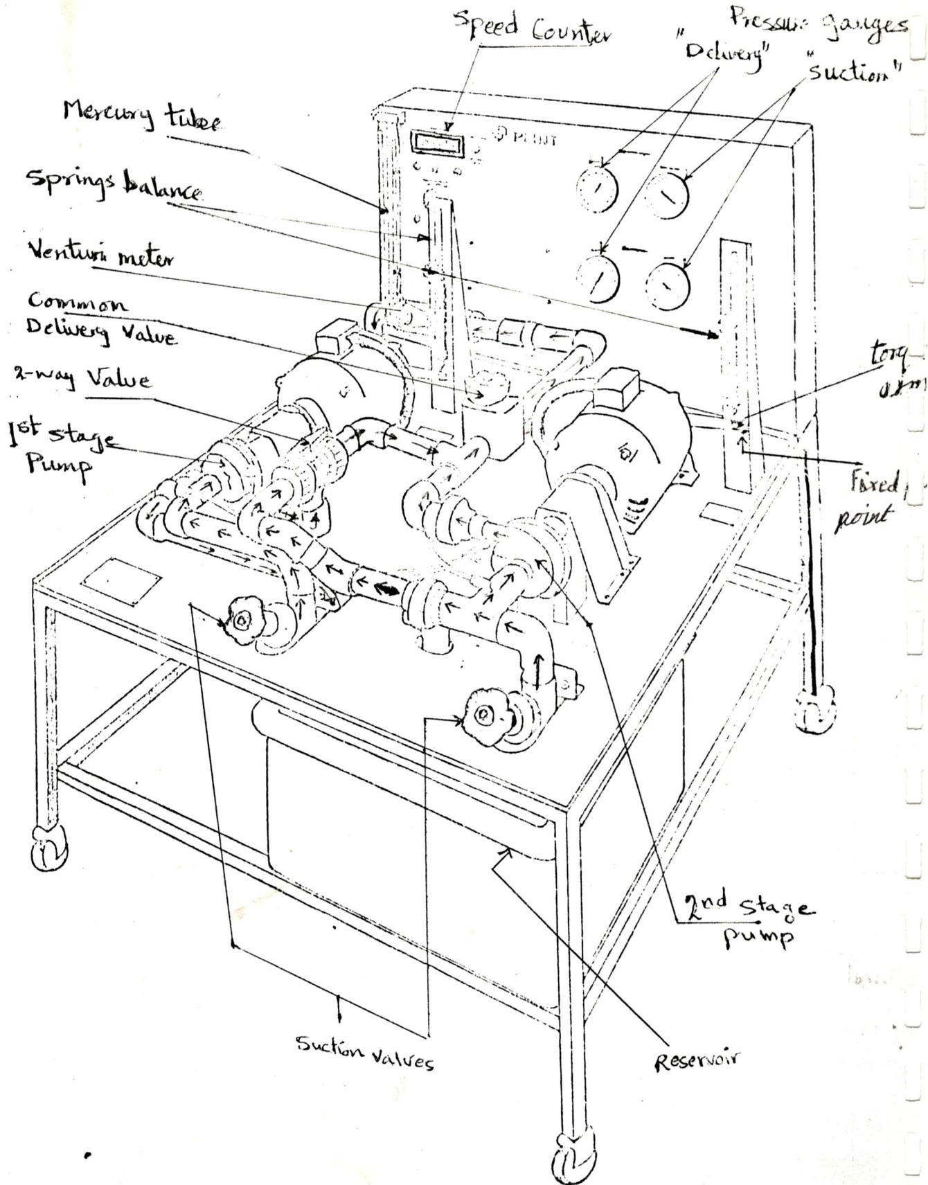
Figure (I) Two Stage Centrifugal Pump Test Set.
