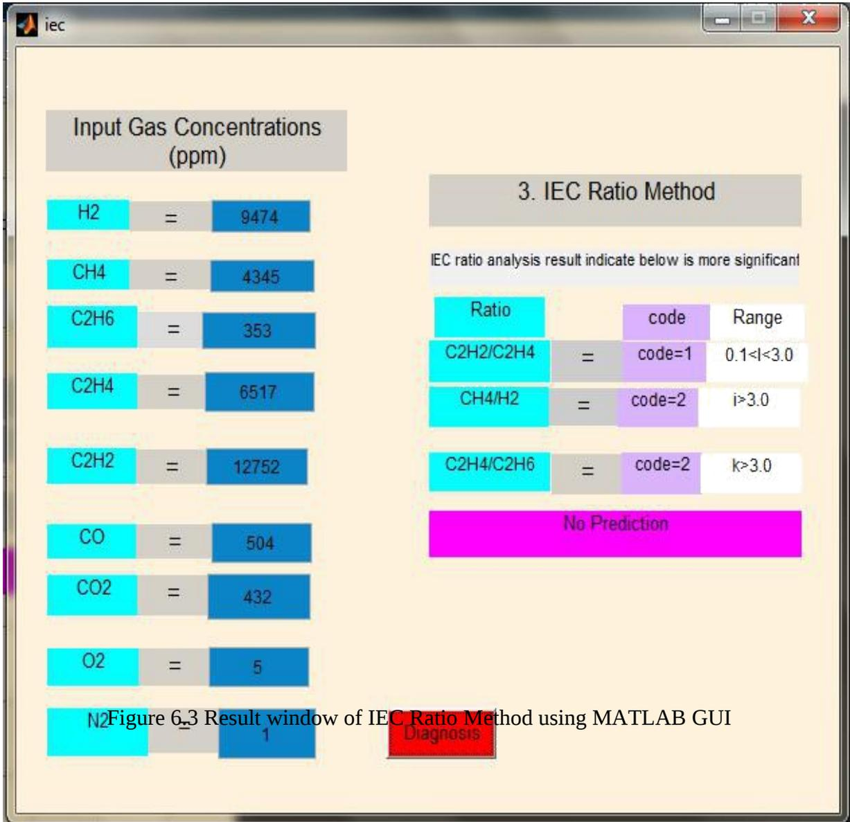
Figure 6.3 Result window of IEC Ratio Method using MATLAB GUI
