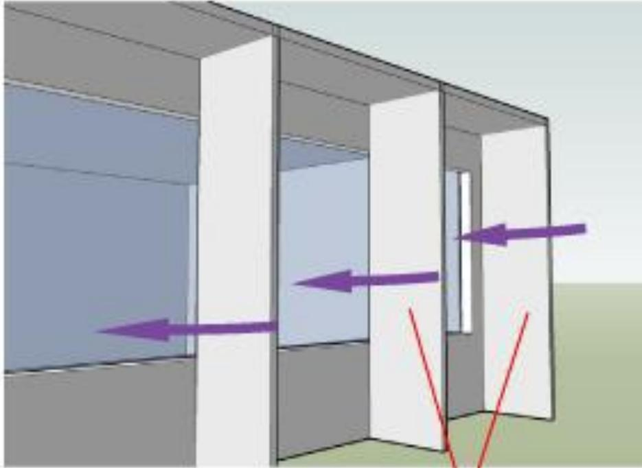
Vertical wing walls can block wind from one direction while admitting wind from another direction, while channeling it into a window opening.
