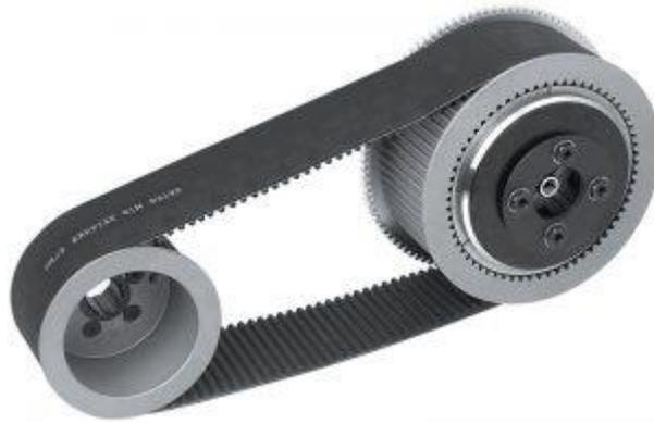
Belt drives are used to transmit power between two shafts which do not have a common axis. The amount of power transmitted between the shafts is dependent upon the amount of friction between the two. Factors that determine the power transmission are the velocity of the belt, belt tension between the pulleys and the angle of contact between the pulleys.
