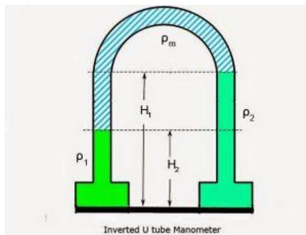
The equation for the same (source: <http://www.msubbu.in/ln/fm/Unit-I/InvertedUtubeMano.htm>)
