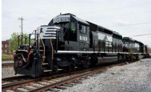
If you notice the shape of the wheel of a train, you will notice that they are conical in shape. The side with greater diameter is on the inside. The shorter diameter lies towards outside. When the train approaches a curve, and has to turn then the wheels slide away in the correct direction. This keeps the train on the track and allows for proper negotiation of the curve.
