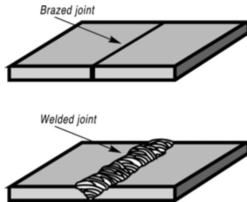
In brazing, only the filler metal is melted to make a joint between the two metals. The wetting is formed between the metals to be joined together and it gets solidified, resulting in a stronger joint. The filler metal goes between the close-fitting parts by capillary action. Brazing is similar to the soldering process. Through these statements, we can say that in **welding** both base metal and filler metal are melted whereas in brazing process only filler metal is melted to make a joint.
