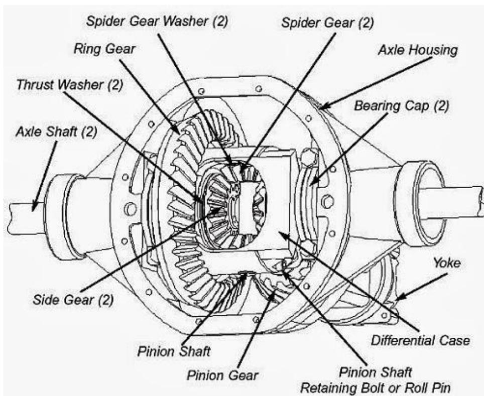
The main function of the differential gear is to allow the drive wheels to turn at different RPMs while both receiving power from the engine. The differential has three jobs:
