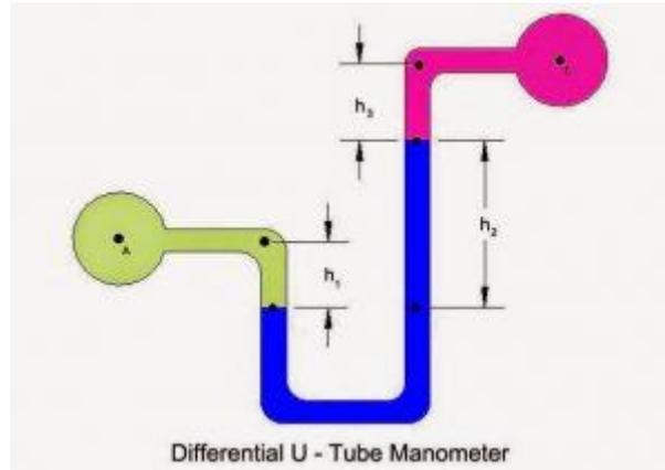
This type of manometer is slightly different from the normal U Tube manometer. Here the open end is also closed, what that means is both the ends of this type of manometer are closed. It really becomes a tool of importance where the pressure is to be measured directly. This manometer type has fluid or liquid filled at different pressures on both ends.
