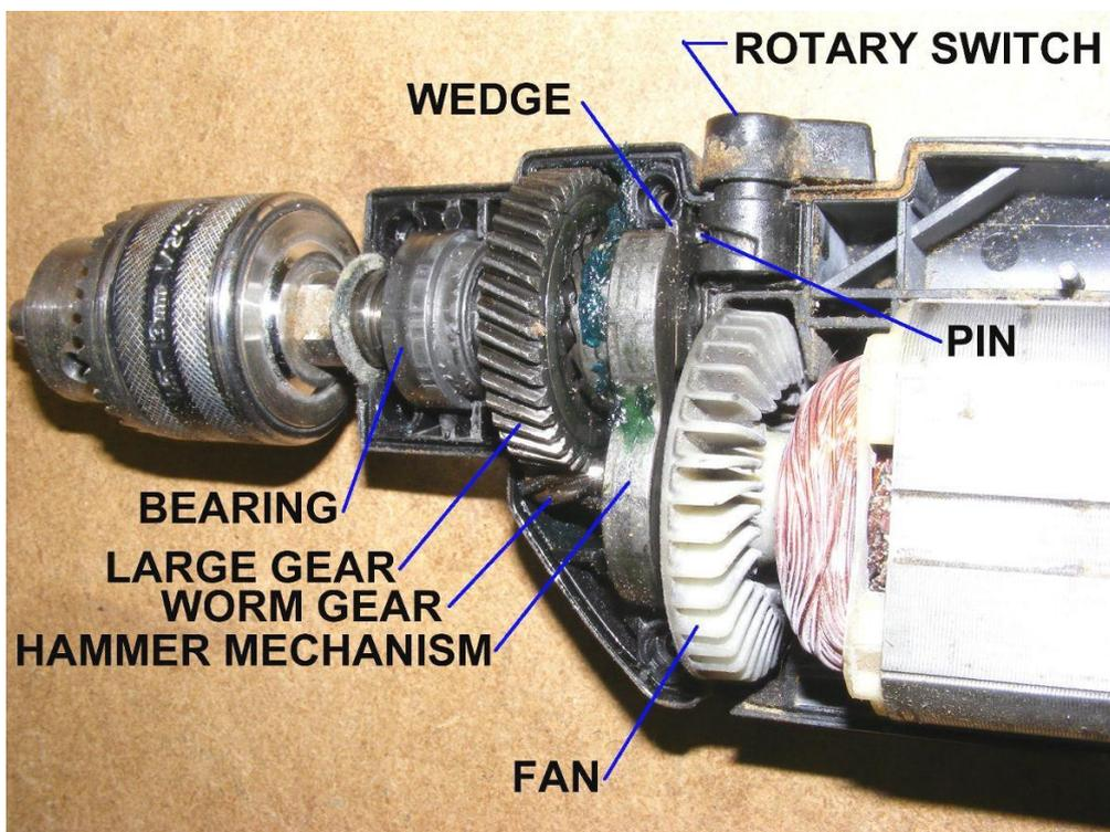
When you turn the rotary switch to impact drill mode it will engage a pulsating gear to the drill spindle and make the drill bit to move forward and backward towards the wall, which works like a chisel while it rotates to break the stone and hardened cement.
