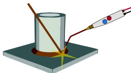
In **welding**, a high temperature is required to melt both base metal and filler metal, but in **brazing**, the temperature is low as compared to the **welding** process.
