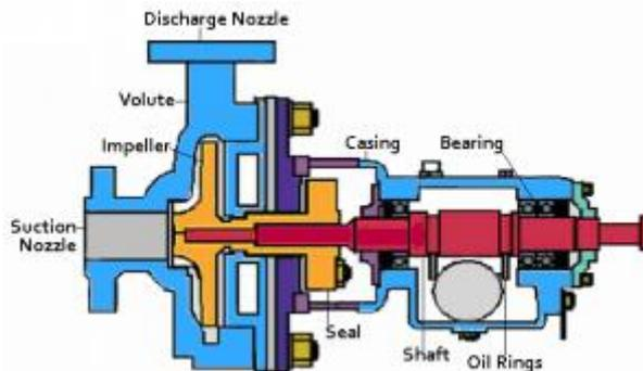
The basic principle of centrifugal pumps is the conversion of rotational kinetic energy to hydrodynamic energy of fluid movement. The fluid enters through the pump impeller near the rotating axis and gets accelerated reaching the desired destination.
