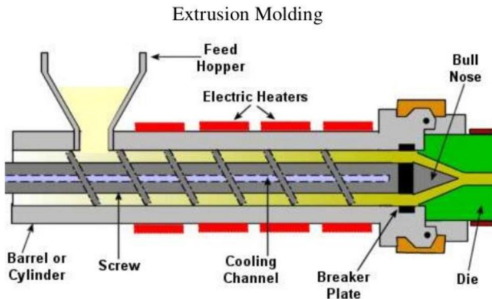
The formed plastic cools under blown air or in a water bath and hardens on a moving belt. Rods, tubes, pipes, Slinkys, and sheet and thin film (such as food wraps) are extruded then coiled or cut to desired lengths.
