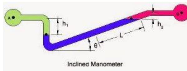
If the manometer, instead of being vertical, is set at an angle  $\theta$  to the horizontal, then a pressure difference corresponding to a vertical difference of levels  $x$  gives a movement of the meniscus  $s = x/\sin\theta$  along the slope.
