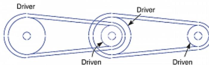
As the name suggests, compound belt drive is a complex arrangement of shafts and pulleys where power is transmitted from more than one shaft utilizing a number of pulleys. It is generally used in a complex application environment.
