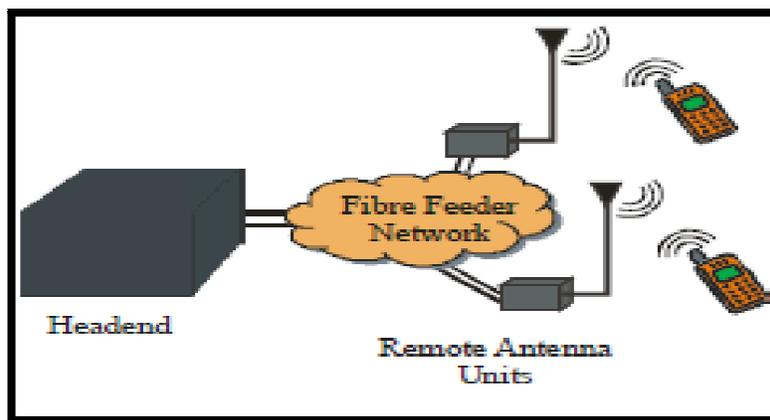
**Figure 2-5:** The Radio over Fiber System Concept
