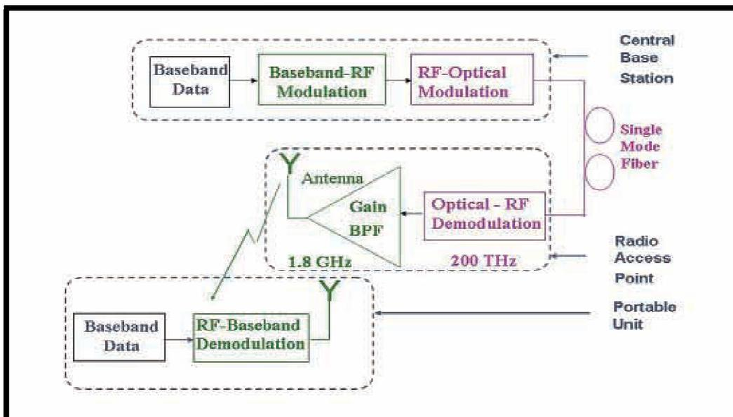
Figure 2-6: Two types of modulation involved with the radio-over fiber
