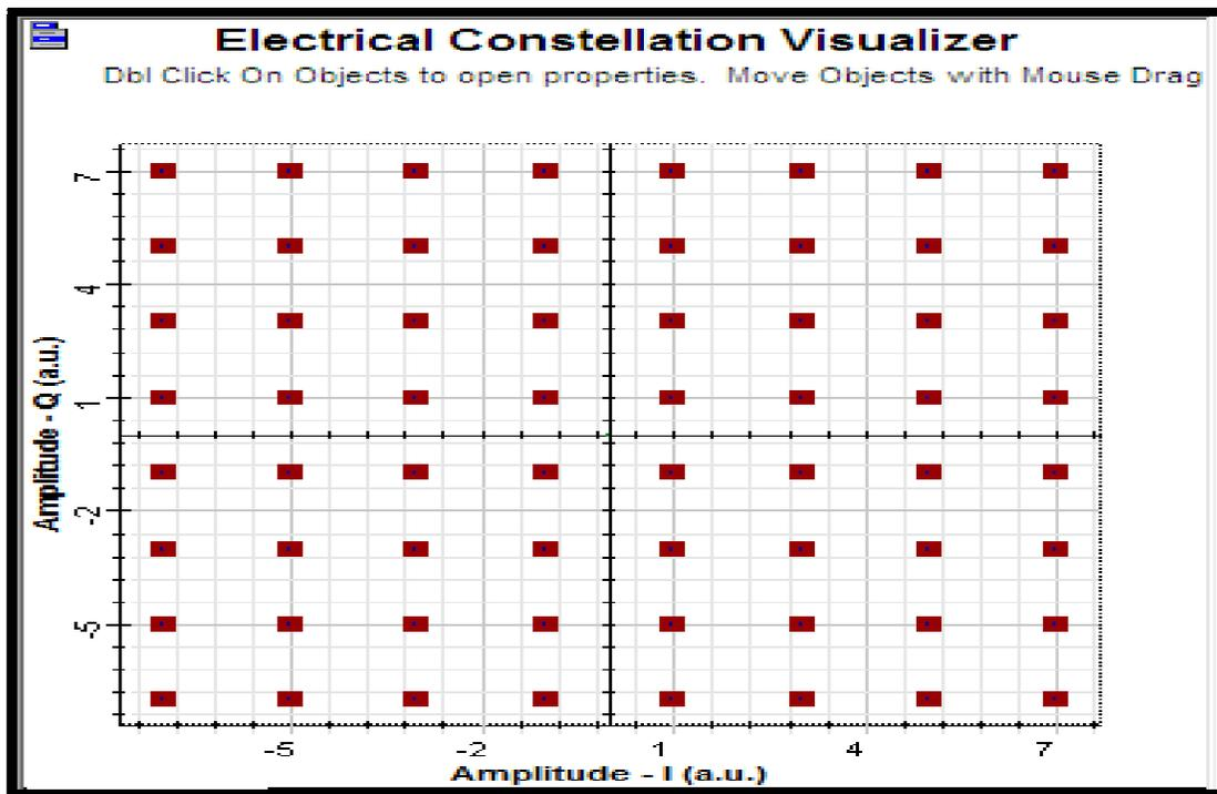
Figure 4.14: QAM constellation diagram
