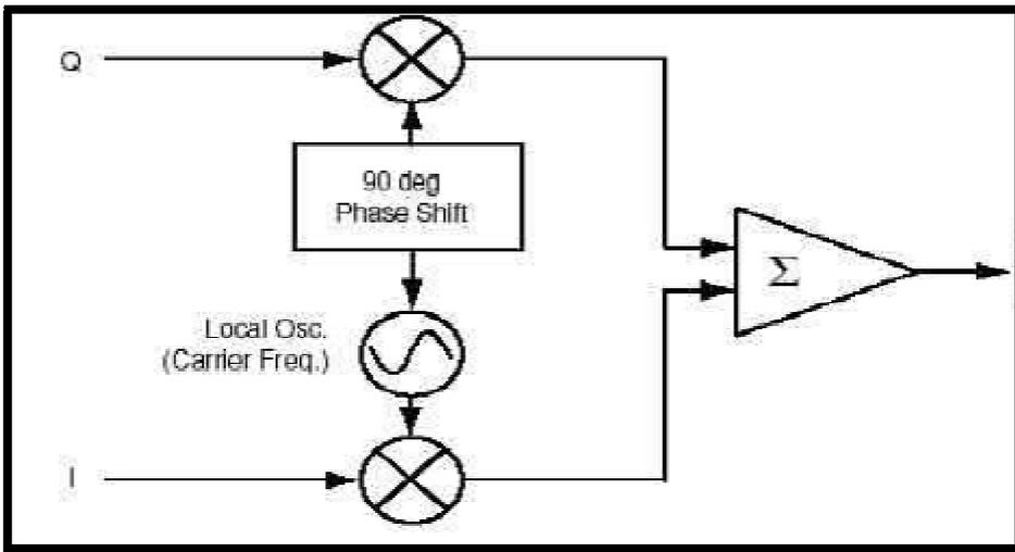
**Figure (3-2):** QAM Modulator
