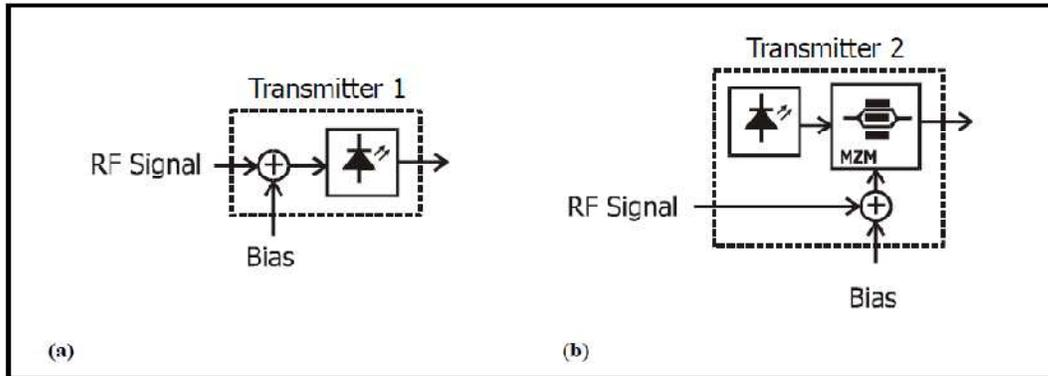
**Figure 2.7:** Generating RF Signals by Direct Intensity Modulation (a) of the Laser, (b) using an external modulator
