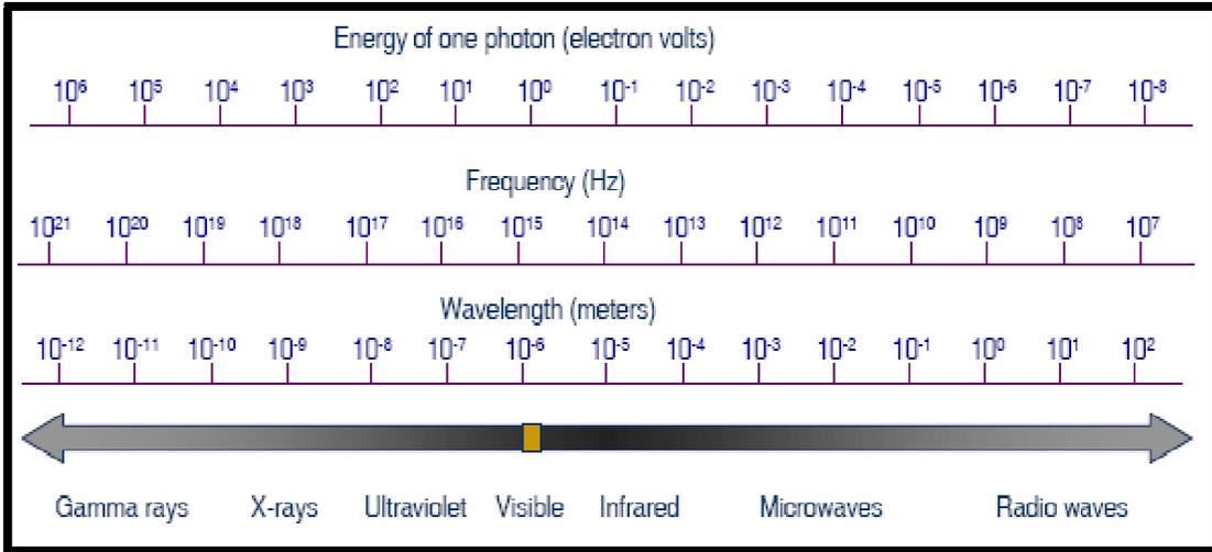
**Figure 2-2:** The radio frequency spectrum
