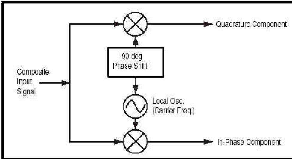
**Figure (3-3):** QAM demodulator
