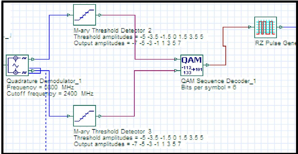
Figure 4-4: Demodulation of electrical signal in uplink
