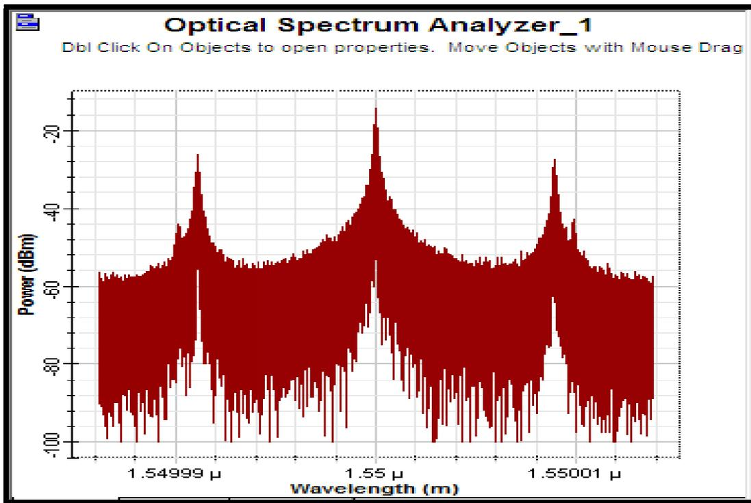
Figure 4-15: Modulated optical signal
