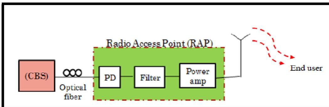
**Figure4-2:** Radio Access Point
