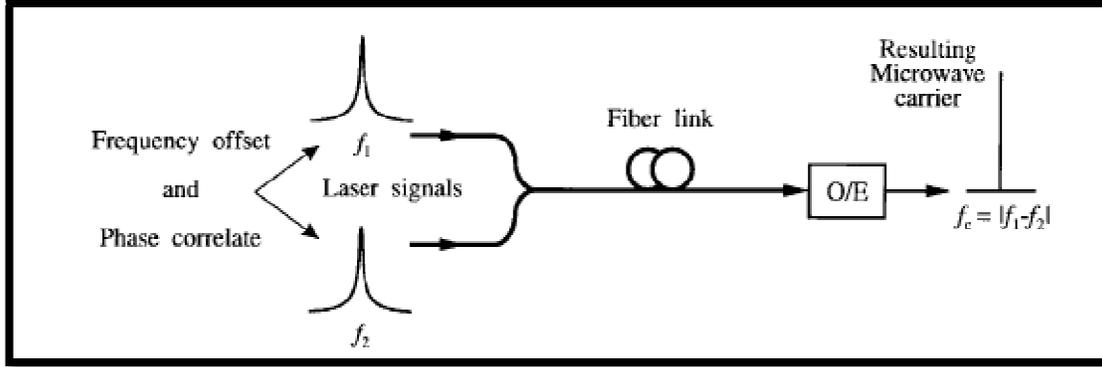
**Figure 2.8:** Remote Heterodyning Detection (RHD) techniques.
