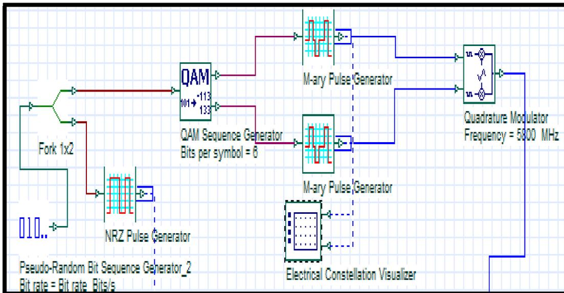
**Figure 4-3:** Generating electrical signal in downlink
