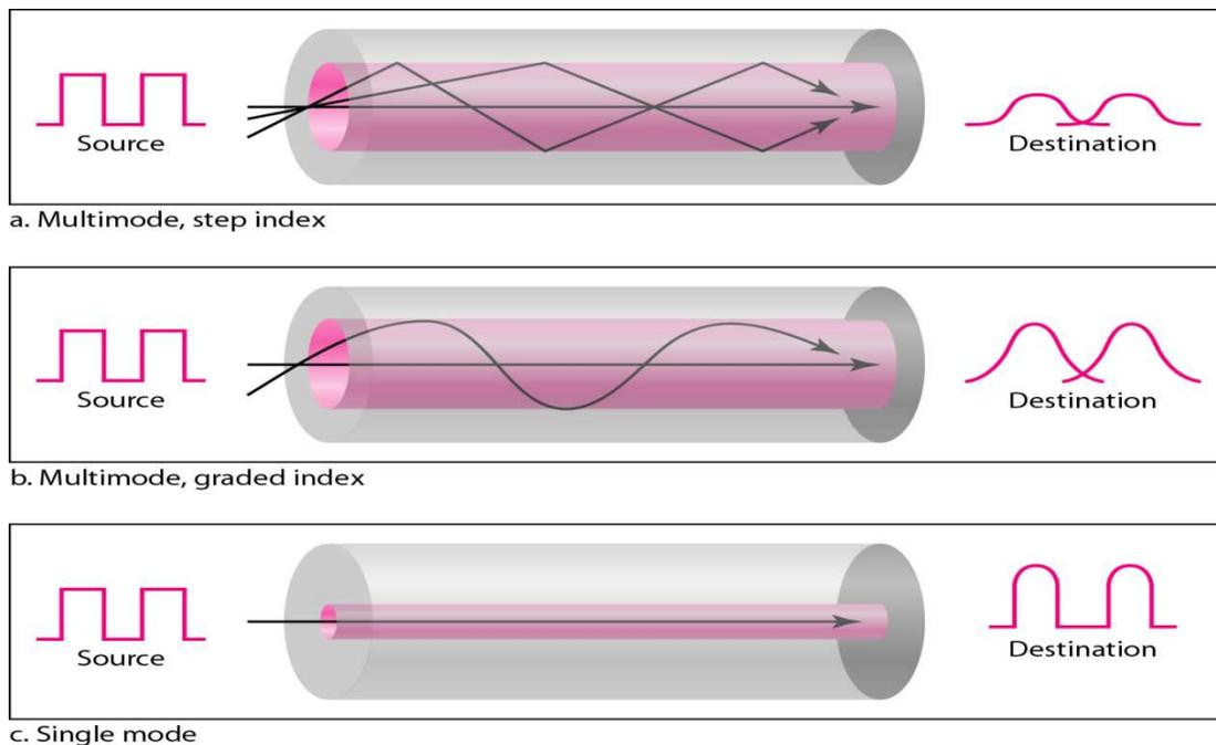
**Figure 2-4:** Optical Fiber types
