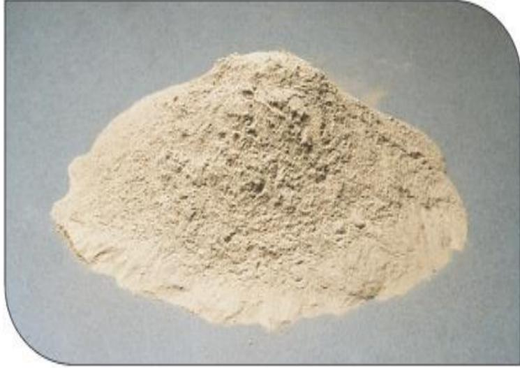
Figure 1. Fly ash, a powder resembling cement, has been used in concrete since the 1930s. (IMG12190)
